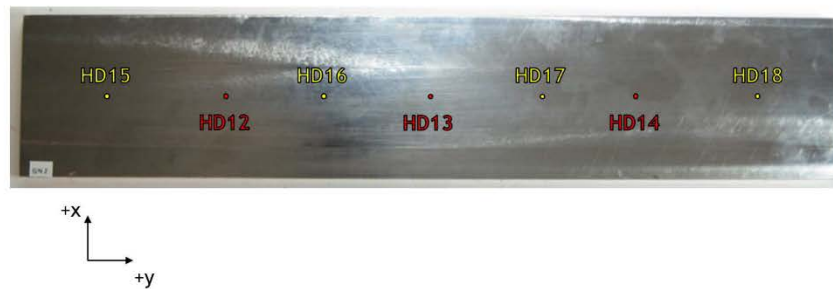
Figure 3: Representative diagram of hole drilling measurement locations for specimens: SN 1 and SN 2.
